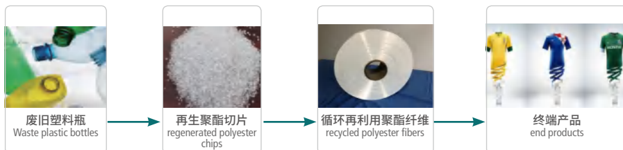
制备流程图 Flow Chart of Preparation
