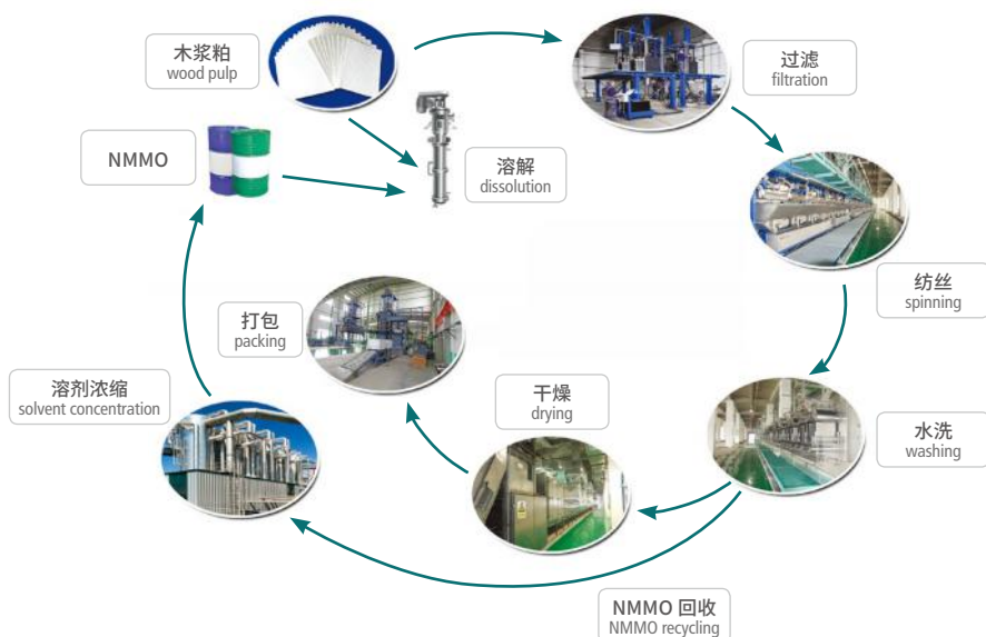
流程示意图 Flow Chart of Preparation
